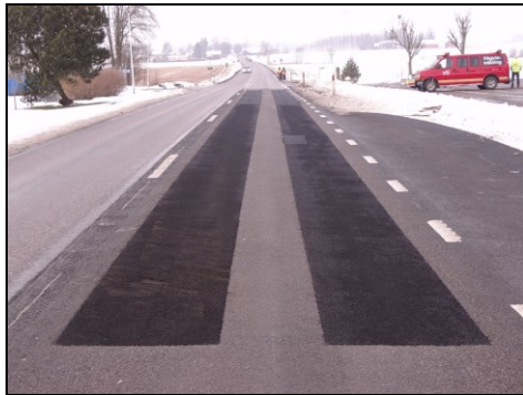
Figure 13: Swedish full scale test tracks in Sjögestad in February 2016, i.e. 1,5 years and two winters after construction. The Sjögestad II surface with the PERS prefab panels (applied only in both wheel tracks) can be seen on the foreground. Note some scars by the snowplough and some raveling. The slightly lighter colored PERS surface in the background the original in situ constructed PERS test track (Sjögestad I)
