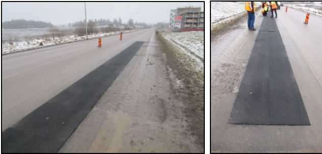
Figure 12: Swedish full scale test track constructed with PERS prefabricated slabs in Linköping in February 2014 (PERS slabs only applied in the right hand wheel track)
